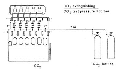
At least two bottles ought to be installed. In most cases, one bottle should be sufficient to extinguish fire in three cylinders, while two or more bottles would be required to extinguish fire in all cylinders
