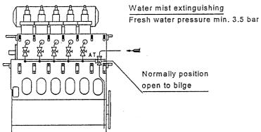
To prevent the fire from spreading to the next cylinder(s), the ball-valve of the neighbouring cylinder(s) should be opened in the event of fire in one cylinder
