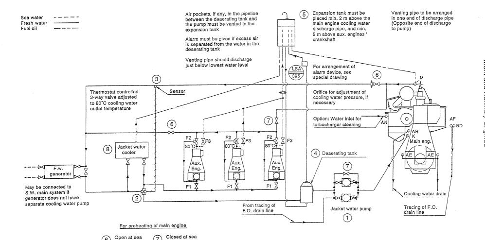
When preheating a stopped aux. engine from running aux. engine, hot cooling water will be led into stopped engine at "F3" and out at "F1"
